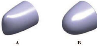
Figure 17: The Bows profiles; tango shape (A) and standard shape (B)
