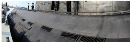
Figure 15: Free board, deck and free flooding space in submarine
